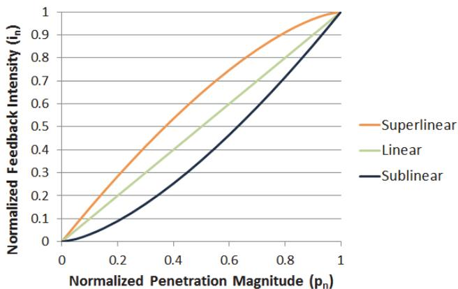
Fig. 3. Mapping functions. Values are normalized such that 1 represents maximum value for interpolation range and feedback effect magnitude. Sublinear is  $i_n = p_n^{1.5}$  and superlinear is  $i_n = 1 - (1 - p_n)^{1.5}$ .
