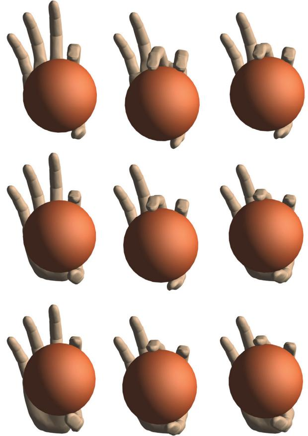
Figure 1: Grasped object positions and virtual hand behavior. Columns, left-to-right: 2-digit grasp, 3-digit with fixed coupling, and 3-digit with adaptive coupling. Rows, top-to-bottom:  $m = 1$ ,  $m = 2$ , and  $m = 4$ . Viewpoint and tracked hand configuration are constant, except tracked middle finger configuration, which is identical for all 3-digit grasps.
