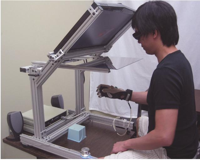
Figure 2: VR equipment with mirror-based display.
