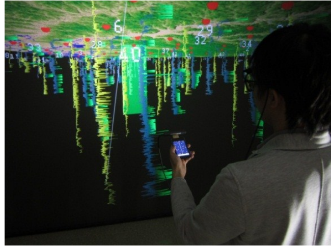
Figure 2: Application used in the experiment. It shows well logs (target objects) creating a dense virtual environment. The user is holding a tracked iPod touch interface.
