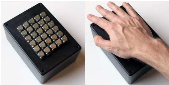
Fig. 1. The vibrotactile array used in our experiment. Six rows of five pager motors are mounted on a project box containing a controller. The array is commanded via serial communication with a host computer.
