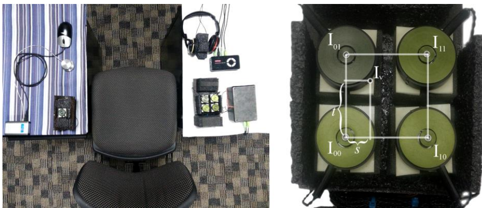
Figure 2: Apparatus. Left: Subjects sat between two devices, placing an arm on each. Right: Four C2 Adjustment Factors labeled with per-factor intensities I_{st} and interpolation parameters on a unit cell. The contribution of I_{00} to virtual factor intensity I_v is determined by interpolation parameters s and t .
