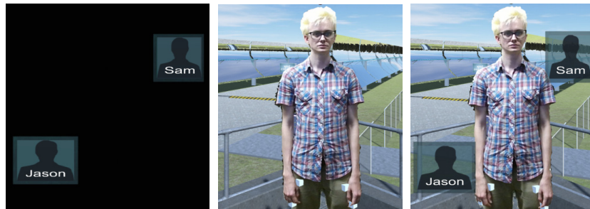
Fig. 5. Gaze targets. Left: overlay rendering. Middle: main scene. Right: composed result. The teacher looks at an indicator to make eye contact with that student.
