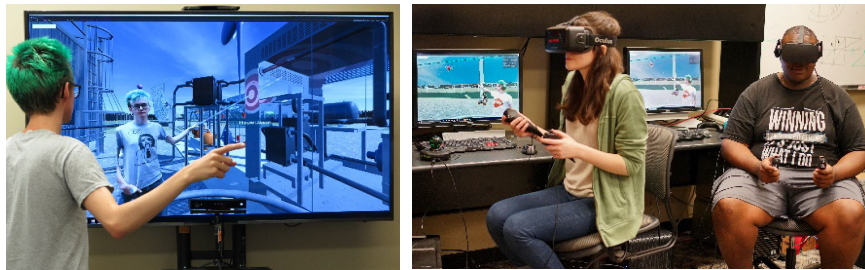
Fig. 1. Teacher guides students in an educational application. Left: teacher points in front of a TV with a Kinect depth camera. Right: Students immersed with HMDs (Oculus Rift) and tracked wands (Razer Hydra). Students also wear headsets with microphones (not pictured).
