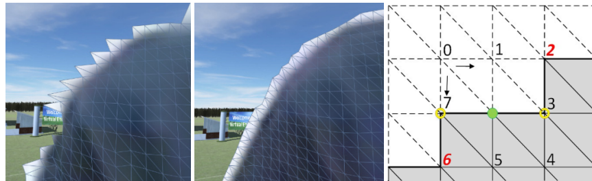
Fig. 4. Mesh edge before (left) and after (middle) refinements. Right: mesh vertices numbered by indices into a MeshUV offset list for accessing them from the central vertex.
